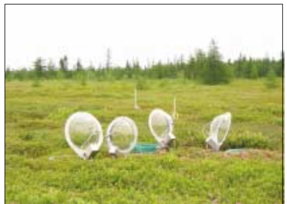
'Auto-chambers' measuring ecosystem exchange of carbon dioxide in the Mer Bleue Bog (Ottawa) for the Fluxnet-Canada Research Network . The data also contributes to the Canadian Global Coupled Carbon Climate Model and helps in evaluating the 'McGill Wetland Model'. CFCAS supports both networks. Photo: D. Conway
